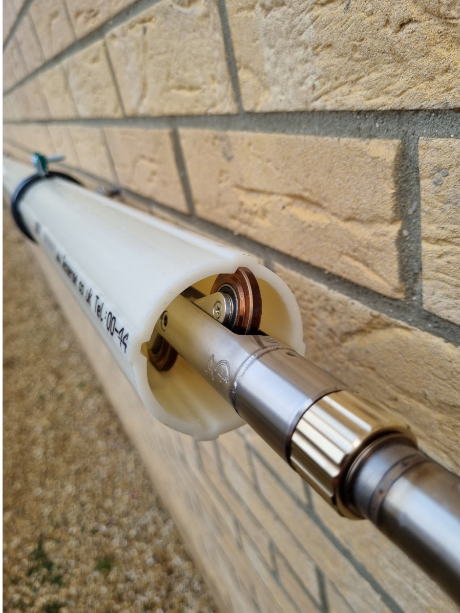
Figure 22: Inclinometer probe inserted into access casing.
