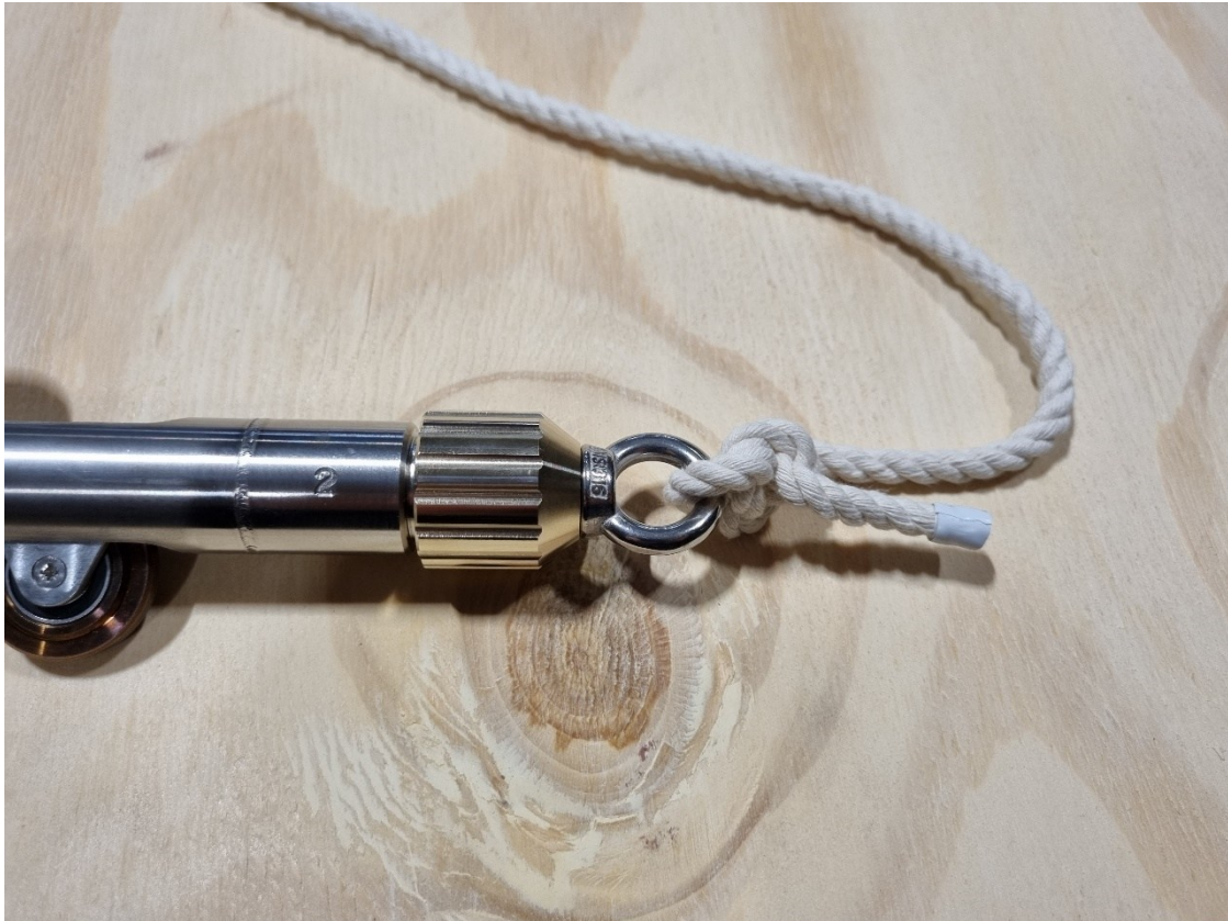
Figure 19: Eyelet cap attached to second end of the probe, marked with 2 rings in later models (a 2 is shown in this model)
