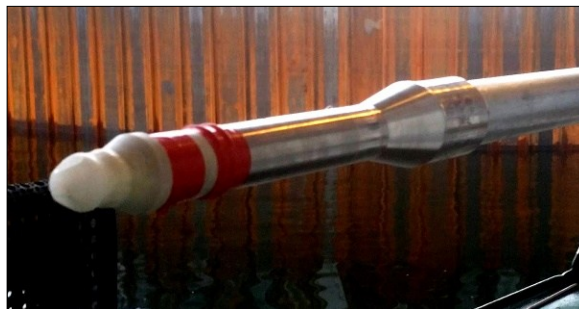
Figure 7: Push-in adaptor for BSP pipe or CPT rods
