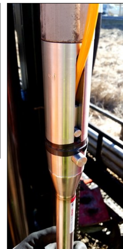
Figure 8: Push-in adaptor for drill rods
