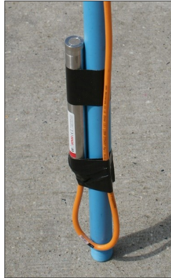
Figure 9: VWP-3000 attached to a PVC tremie pipe
