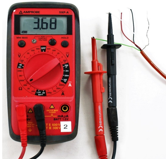
Figure 15: Multimeter measuring resistance across the green and white cores (thermistor)
