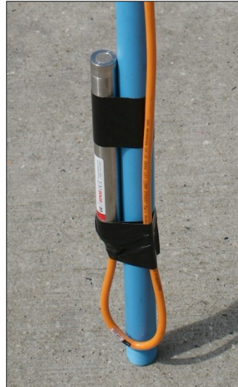
Figure 9: VWP-3000 attached to a PVC tremie pipe
