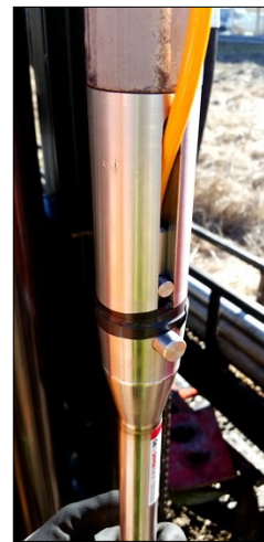
Figure 8: Push-in adaptor for drill rods
