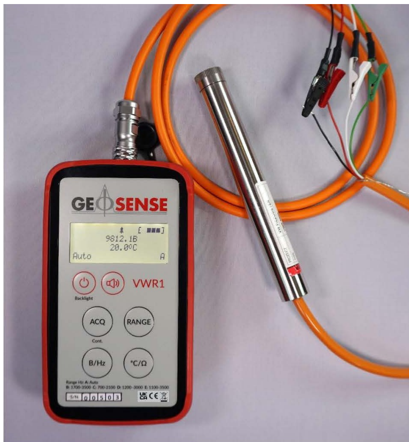
Figure 1: VWR1 with fly lead measuring a Geosense VWP-3000
