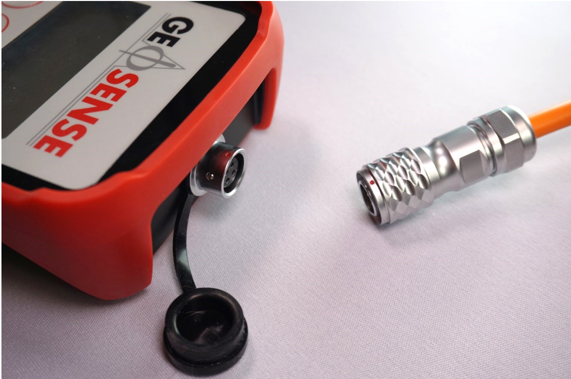
Figure 3: Connector and port showing alignment dots in red
