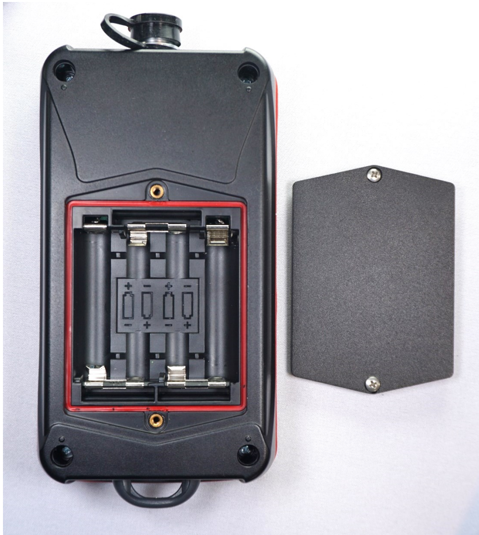
Figure 5: Rear battery compartment of VWR1
