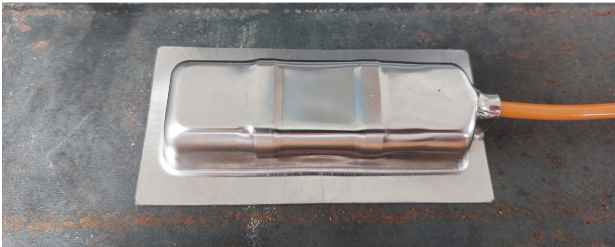
Figure 24: Cover for a spot weldable strain gauge prior to being spot welded onto the structural steel member
