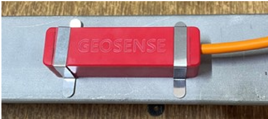
Figure 23: a coil housing with spot weldable straps over it to hold it to the metal (straps awaiting spot welding in this image)
