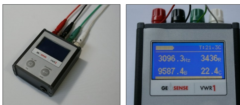
Figure 30: VWR1 connected to vibrating wire sensor with thermistor for temperature
