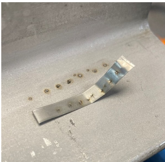
Figure 26: A demonstration of a bad weld where the strip has pulled cleanly off with discolouration to the metal.
