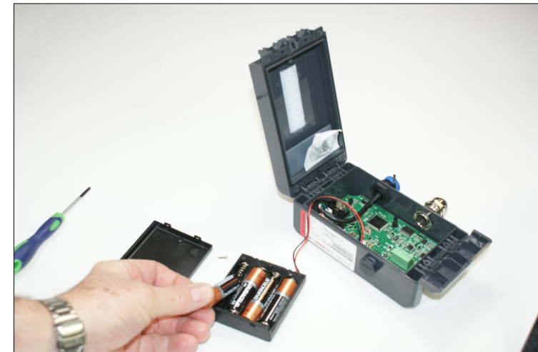
3. Remove the battery holder, undo the screw securing the lid and fit the batteries
