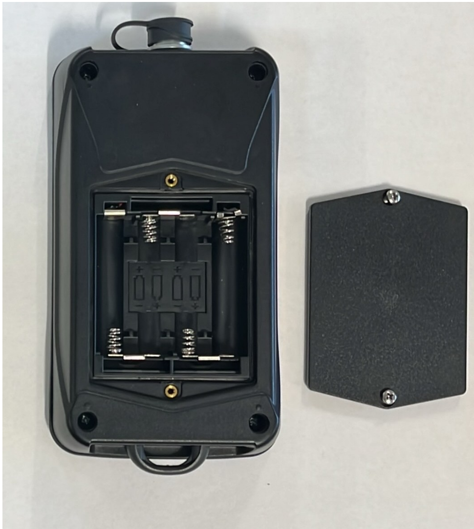
Figure 14: Rear battery compartment of MPR1
