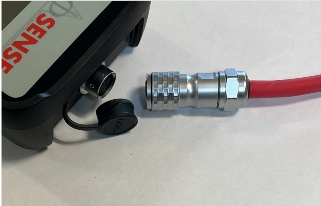
Figure 6: Connector and port showing alignment dots in red
